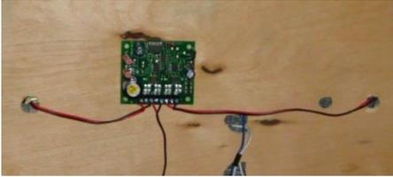
The DS52 can be mounted to the underside of the module top by double-sided foam tape, as shown. The red and black wires extending out each side connect to the two turnouts being controlled. The red and black wires extending down connect to red track power via terminal UniJoiners. Note the DS52 red and black wires could be connected to a separate bus if a suitable bus is available in the layout. The decoder is configured to operate the bi-polar solenoid motors in the Unitrack turnouts.
